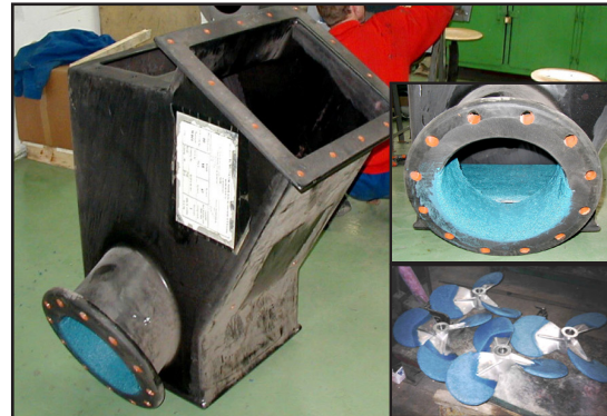
New chutes and mixer blades lined and coated with ARC MX1
